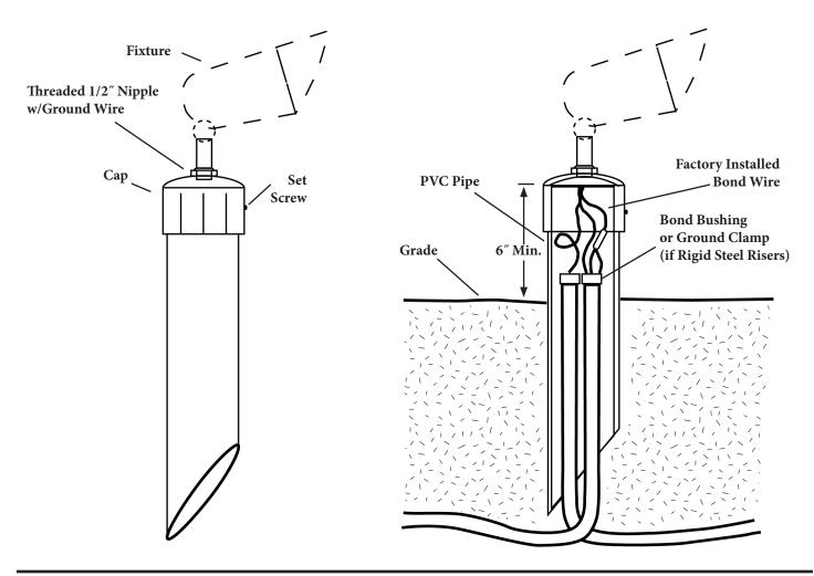
**READ AND UNDERSTAND THESE INSTRUCTIONS BEFORE INSTALLING FIXTURE.** This fixture is intended for installation in accordance with the National Electrical Code and local code specifications. To prevent electrical shock, turn off at fuse box before proceeding.
